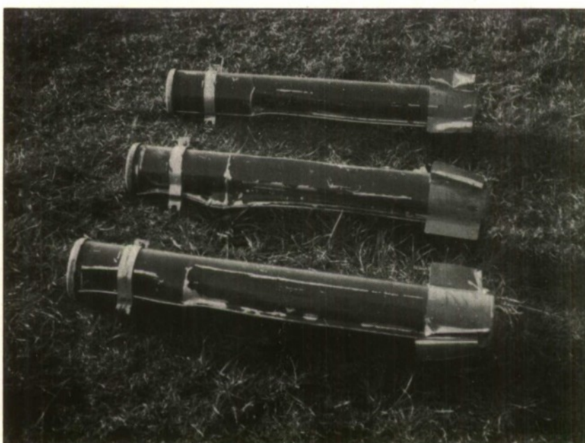
2. 24 S.W.G. (.022) M.S. OUTER CASING LINED WITH SPRUCE AFT AND MAGNESIUM ALLOY SLEEVE CASTING FORWARD
