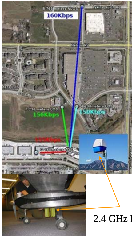
Figure 3 Extended Range ZigBee Connection
