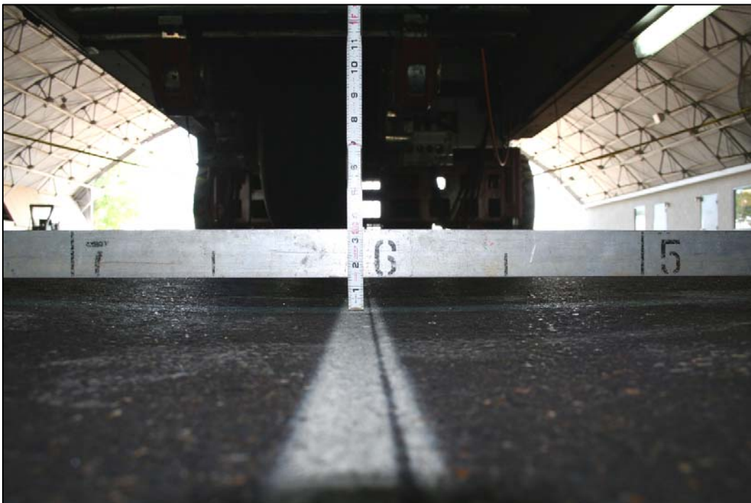
Figure 52. Item 3 rutting after 1,544 passes.
