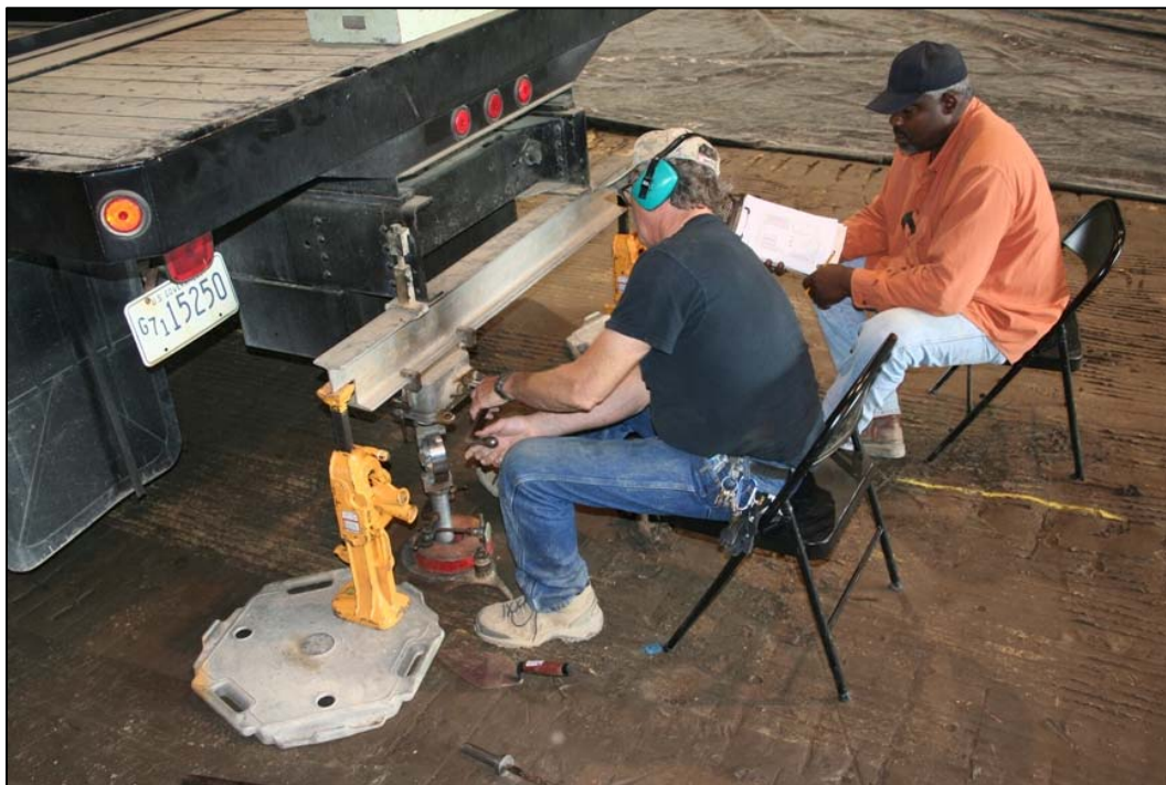
Figure 10. Performing an in situ CBR test on the subgrade.
