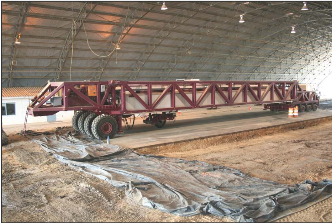
Figure 19. ERDC's HVS-A on the asphalt concrete test section.
