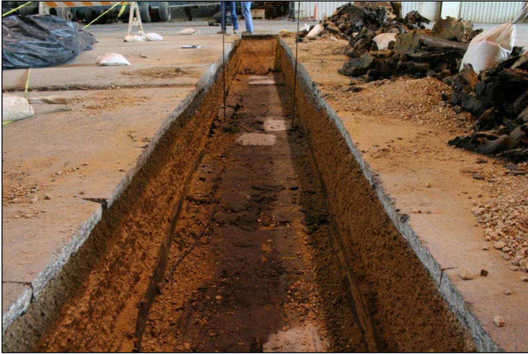
Figure 27. Trench across the center of Items 1, 3, and 5 of the test section.
