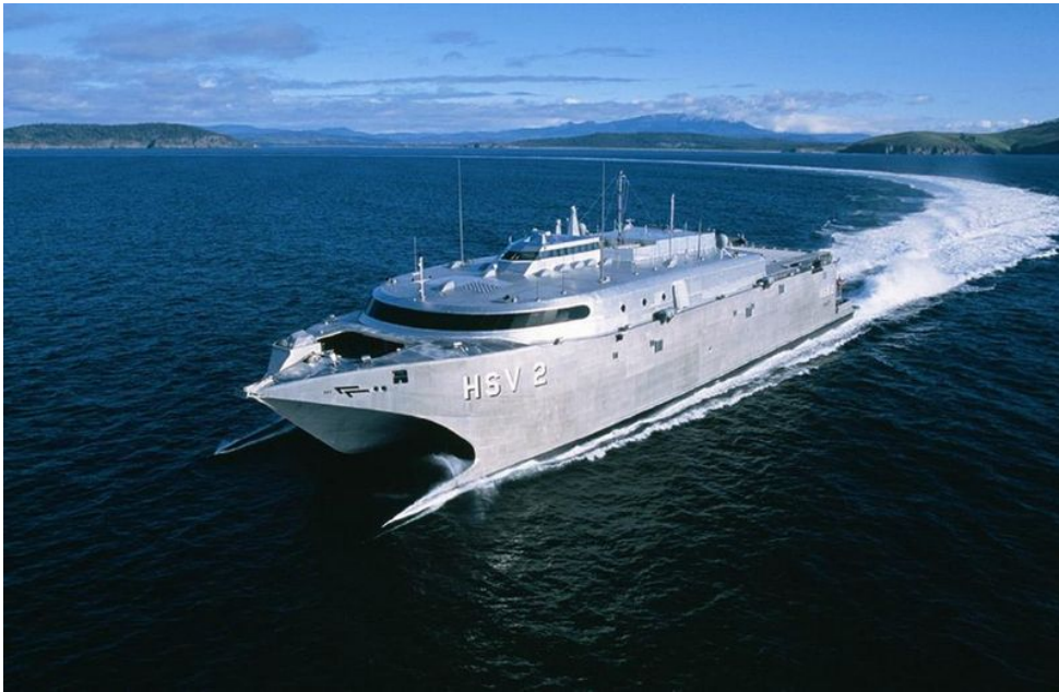
Fig 12: Incat Catamaran with Wave Piercing Bow.
