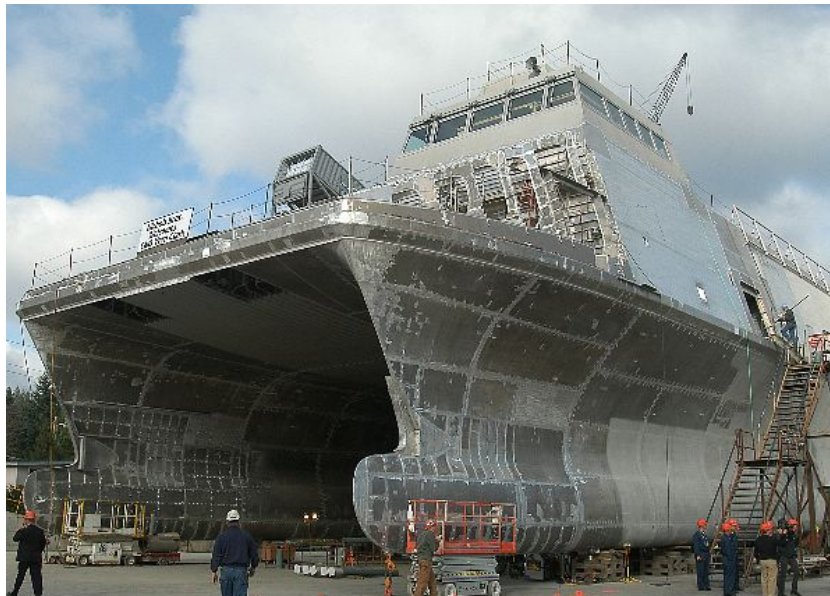
Office of Naval Research high speed, experimental aluminum catamaran “X-Craft”. LOA: 262 ft. long DISP: 950 tonnes(LS) Speed: 50 kts, 40kts in Sea State 4
