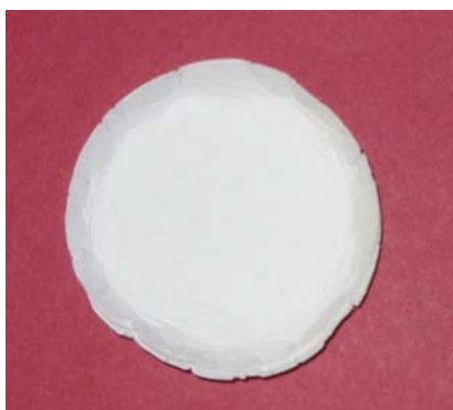
Figure 1. Filtering material after contact with stressed FT fuel.
