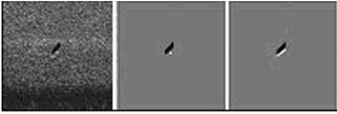
Fig. 5. The image on the left is a sidescan-imagery snippet of a mine-like contact. The middle image shows the results after an adaptive filter was applied to the snippet. The complete shadow of the contact was extracted from the snippet, but the bright spot was not. The completion algorithm uses the shadow to “complete” the bright spot, shown in the image on the right. Attributes, such as height, length and width, are then determined from the “completed” image.
