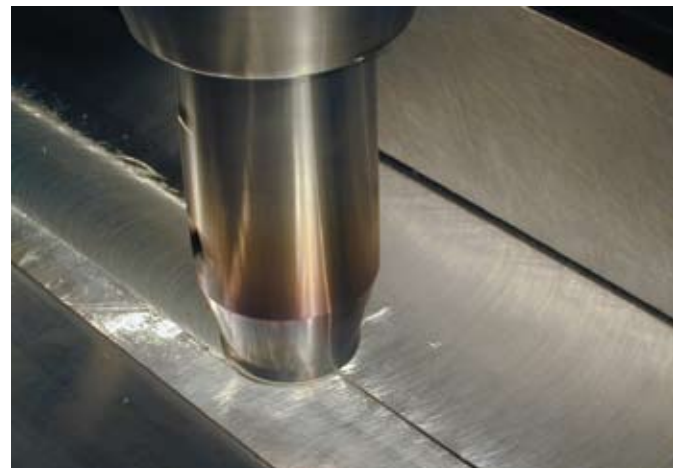
The NCEMT is developing friction stir welding processes for use in U.S. Navy and Army applications.
