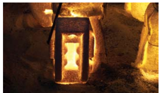
NMC worked to improve the casting process of a stainless steel saddle for Virginia Class Submarines. CTC photo
