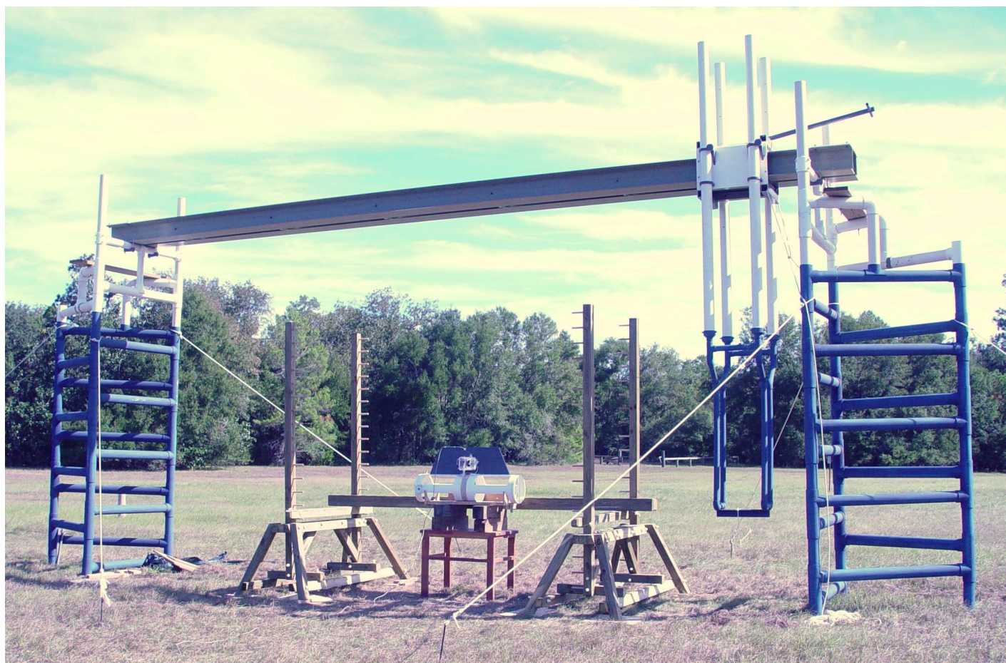
Figure 3. Experimental apparatus used for static and in-motion measurements in our investigation of the GEM53D active electromagnetic sensor.
