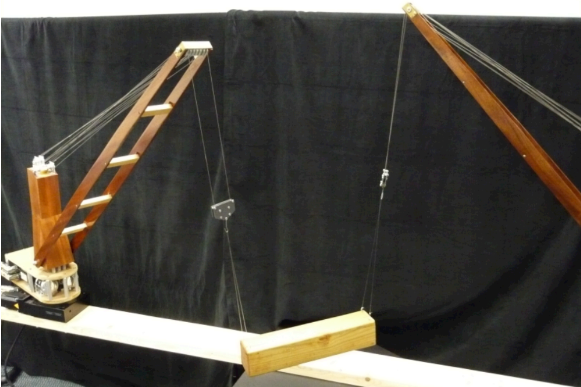
Figure 29. Front view of model of the dual crane system with jibs at arbitrary slew angles. Note the vertical offset of the hoist falls characterized by the angle \rho_I .
