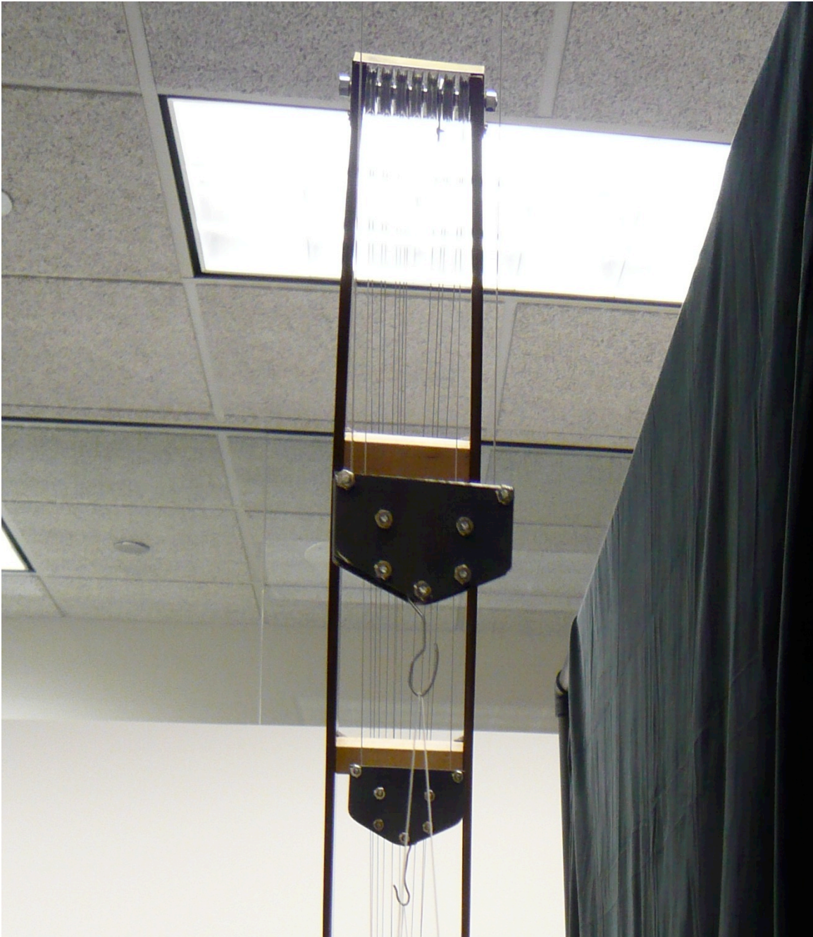
Figure 182. Photograph of jib top of scale crane model showing warping. This warping may produce out-of-plane motion during controlled cases with significant luffing and hoisting motion.
