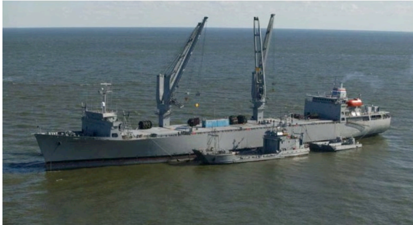
Figure 20. Demonstrating cargo transfer at sea using PCS-controlled luffing-jib cranes on the SS Flickertail State in 2002.
