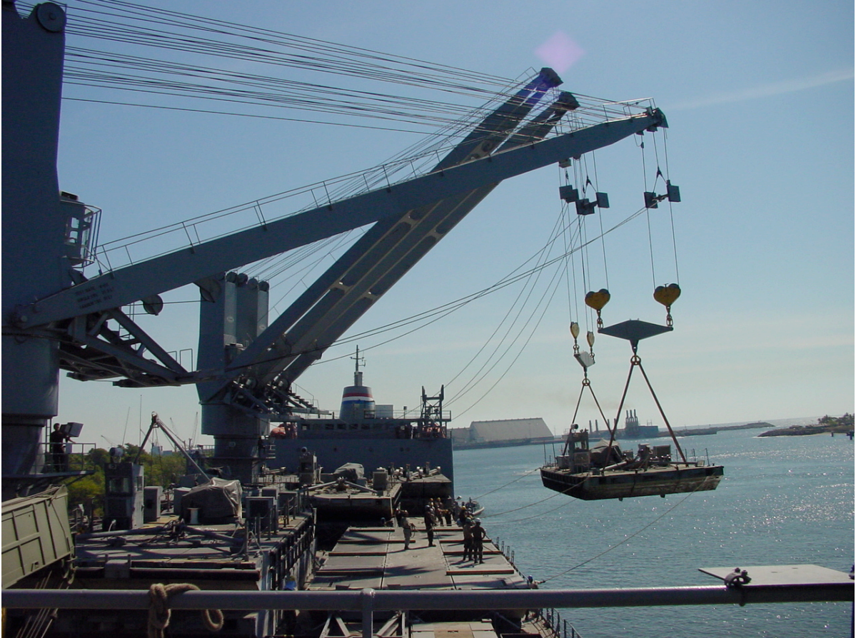
Figure 26. Photo of a U.S. Army modular warping tug being lifted onto the deck of the S.S. Flickertail State by two luffing-jib crane-sets in twin mode during Operation Humanitarian Support Over-The-Shore (HSOTS) 2007 in Puerto Quetzal, Guatemala.
