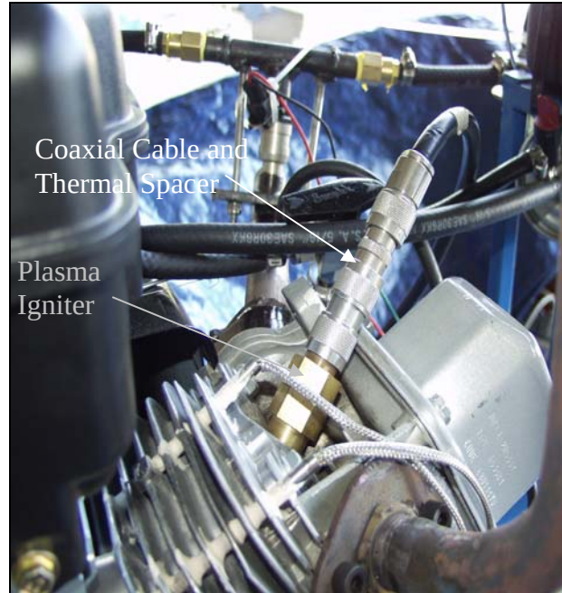
Figure 6. Installed Plasma Igniter
