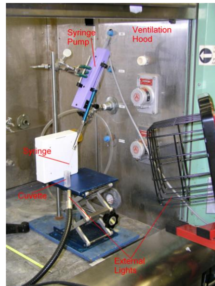
Figure 2. Test Set-up within Ventilation Hood
