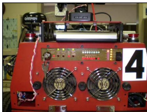
Figure 6. Display panel at ATRV rear.
