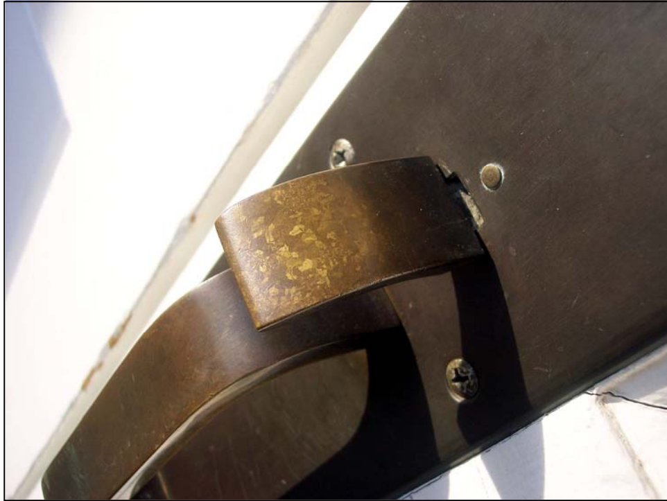
Figure 3. Macroetched brass door handle showing grain structure.
