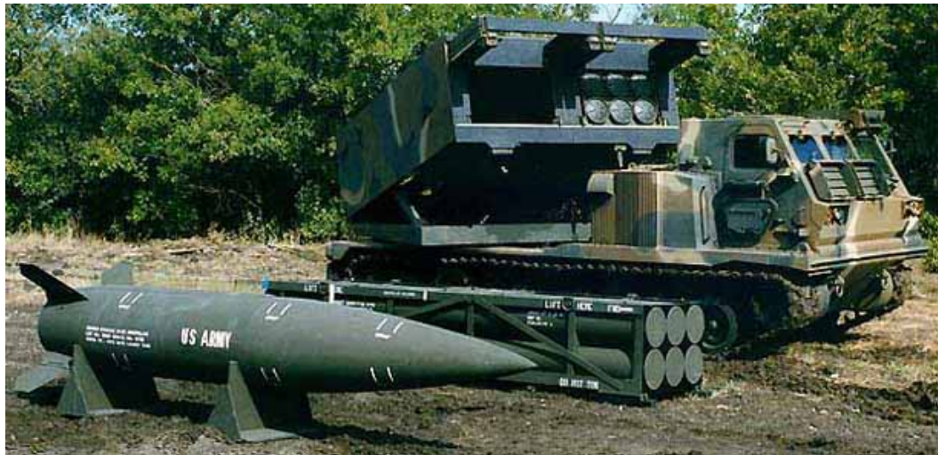
Figure 10. The Army Tactical Missile System Components Launcher, Missile, and Missile Launch Pod Container
