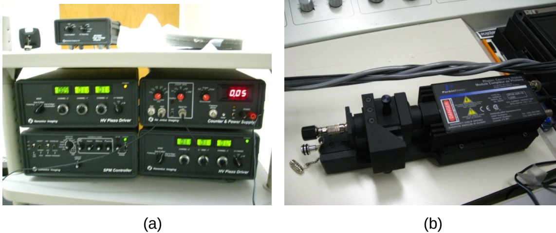
Figure 11 (a) Anticlockwise from Top Left Hand Corner: Low Voltage Adaptor, HVPD for Upper Stage, SPM Controller, HVPD for Lower Stage and Counter and Power Supply for the APD. (b) The APD for Detecting Photons from the Fiber Probe During Measurements.
