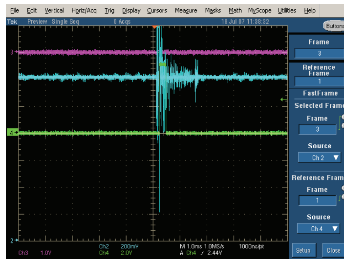
Figure 9. Digital fault pulse (green), diode voltage (red), and optical power (blue).
