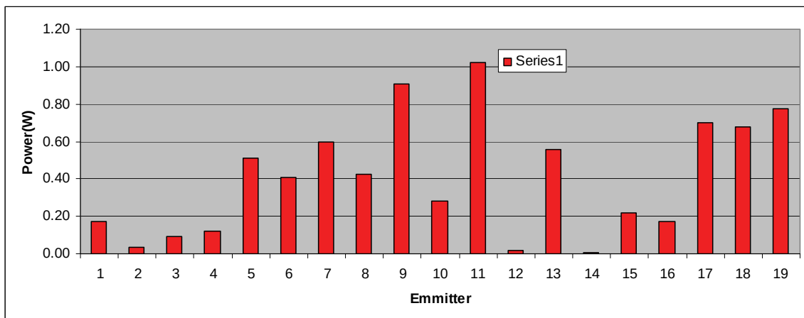
Figure 12. LD41860, post-test power per emitter at 18 A, calculated from figure 10.
