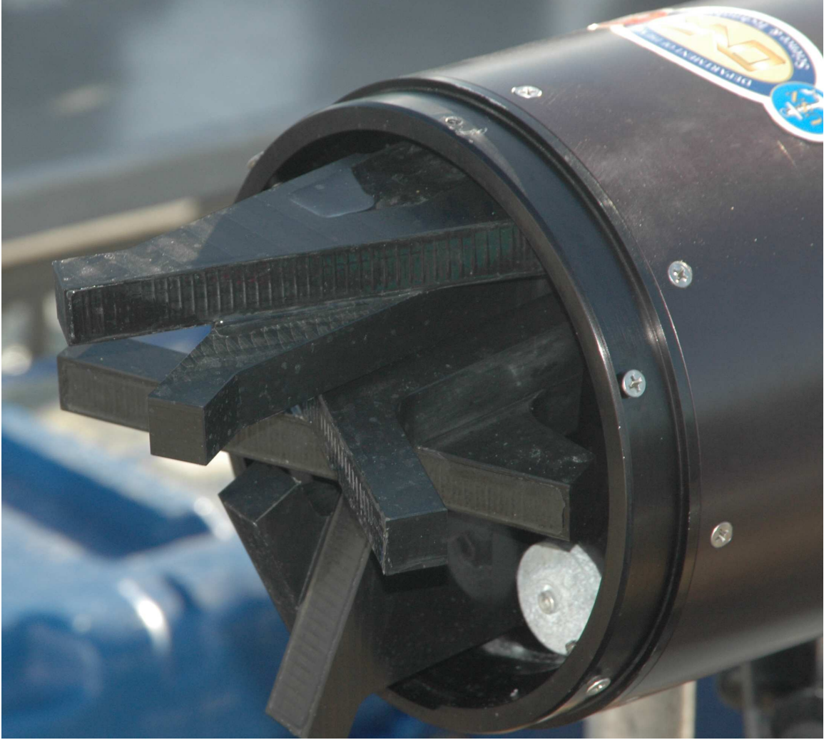
Figure 4. BlueView 450X with nose cone removed to show the six transducer configuration.
