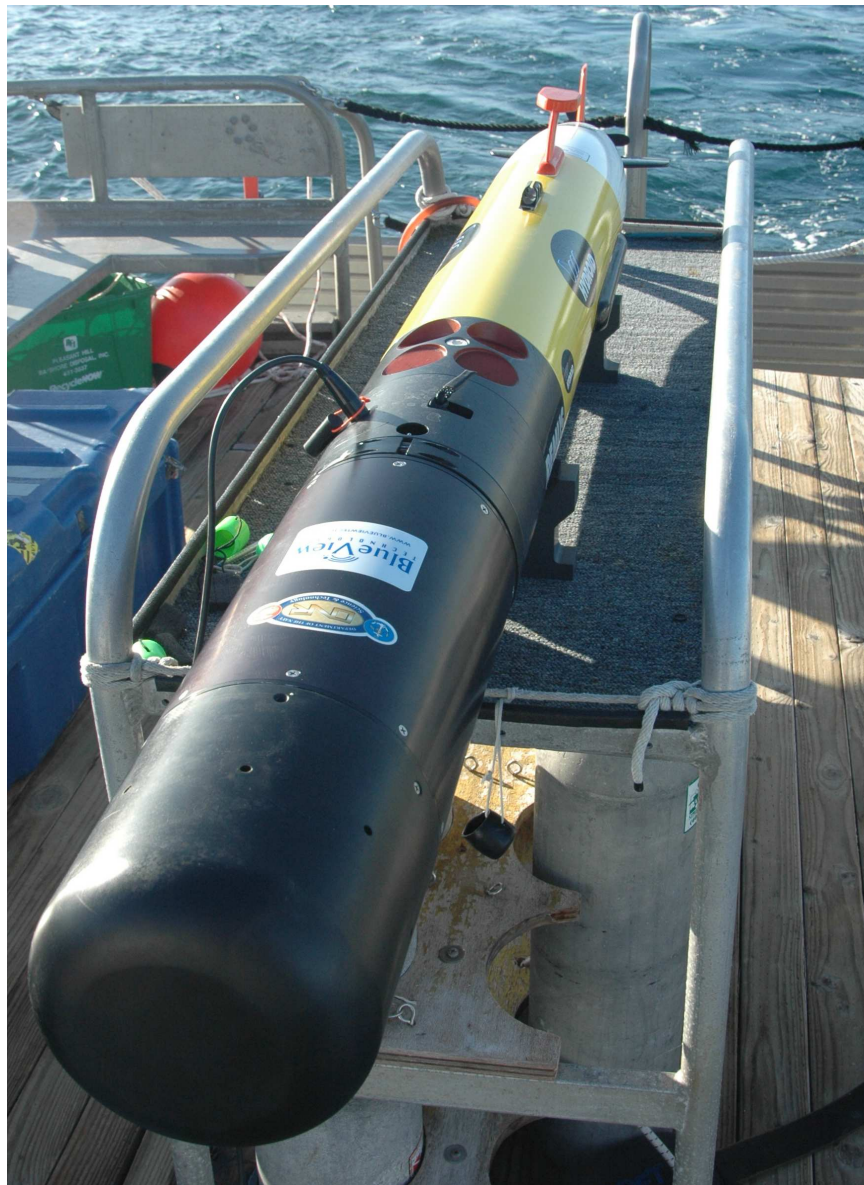
Figure 2. Naval Postgraduate School REMUS 100 AUV with BlueView FLS
