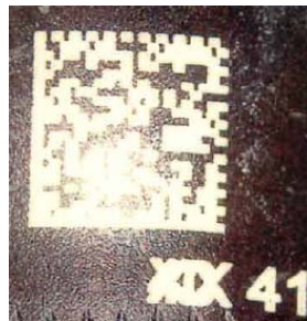
Figure 24. Laser Etch and Clear Coat after Hot, Cold and Icing From (Boyle, 2006)
