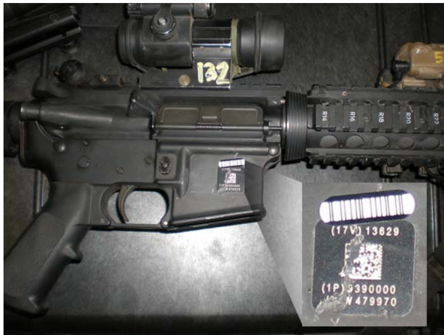
Figure 18. M-4 with damaged UID marking
