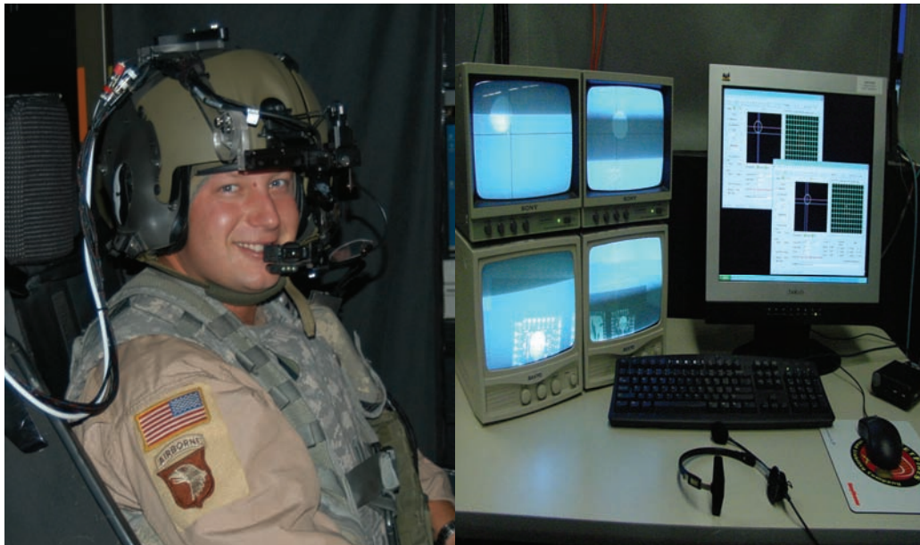
Figure 6. Eye tracker, pupil/camera monitors, and control panel interface.
