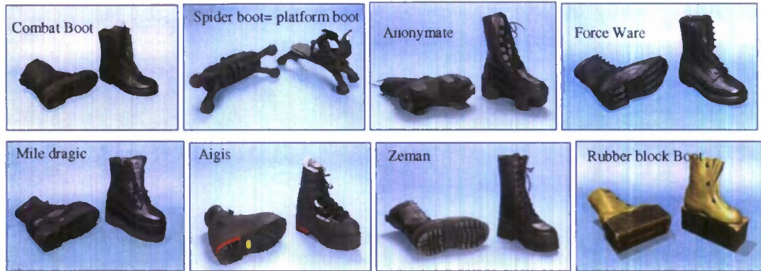
Figure 2 Pictures of the eight mine boots used including the Dutch army combat boot.
