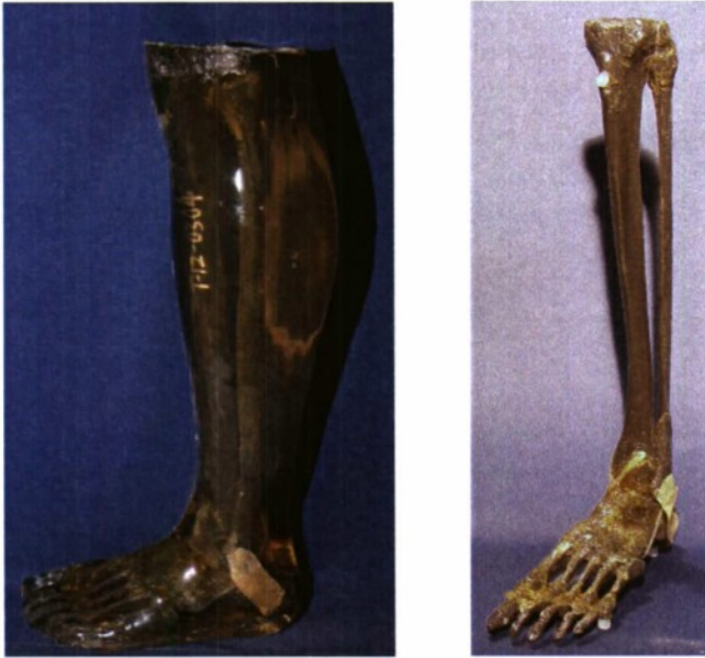
Figure A.4 Left picture shows the FSL cast in gelatin and right picture shows the inner skeleton of the FSL.
