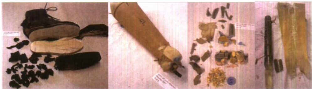
Figure 4 An example (test 5). Boot damage, CLL visual injury assessment. The leg and foot, inspecting the CLL, appear not to be damaged significantly. However when the latex confinement is removed the real severe injury is revealed. The calcar bone, with heel pad and tibia is cracked and fragmented. The foot is amputated. There is soft tissue damage in the lower leg part, just above the ankle. Besides, there is a severely damaged ankle joint. The talus was broke into two main fragments. The calcar bone (rear and front) were both broken into two main fragments and small pieces. The foot sole of the CLL was damaged.
