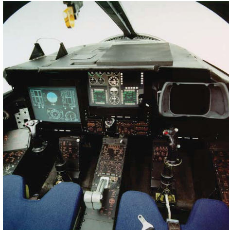
Figure 13: Photograph of an example of a cockpit module. This photograph shows an F-111C cockpit where the main instrument panel has been replaced by three computer monitors which allow for the display of software versions of primary and secondary flight instruments, as well as other types of displays.
