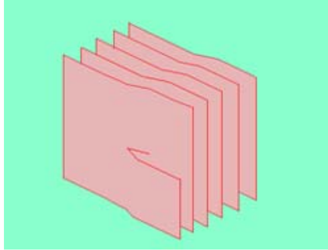
Figure 4. Schematic Diagram Showing a Screw Dislocation [From: 16].
