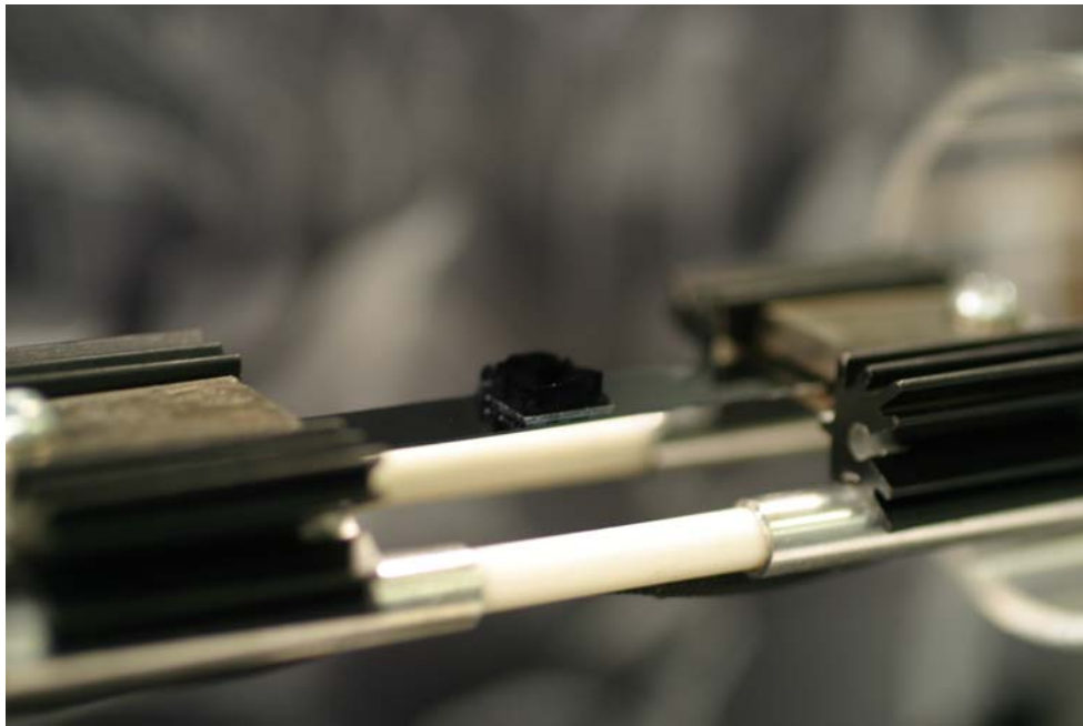
Figure 51: CNT growth in the SabreTube
