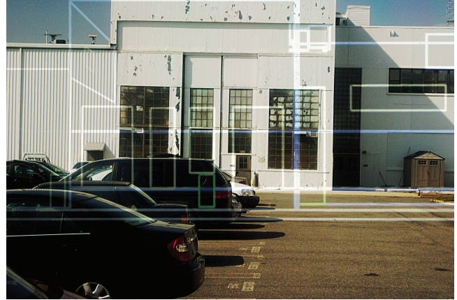
Figure 1: A typical registration error, in which the rectangles that represent the windows, doors, and the building outline are clearly displaced from the correct locations. The low contrast of this image is due in large part to the difficulty of taking a photograph through an optical see-through display. This and similar images in Figures 2, 3, and 4 have been enhanced to improve the visibility of the graphics.
