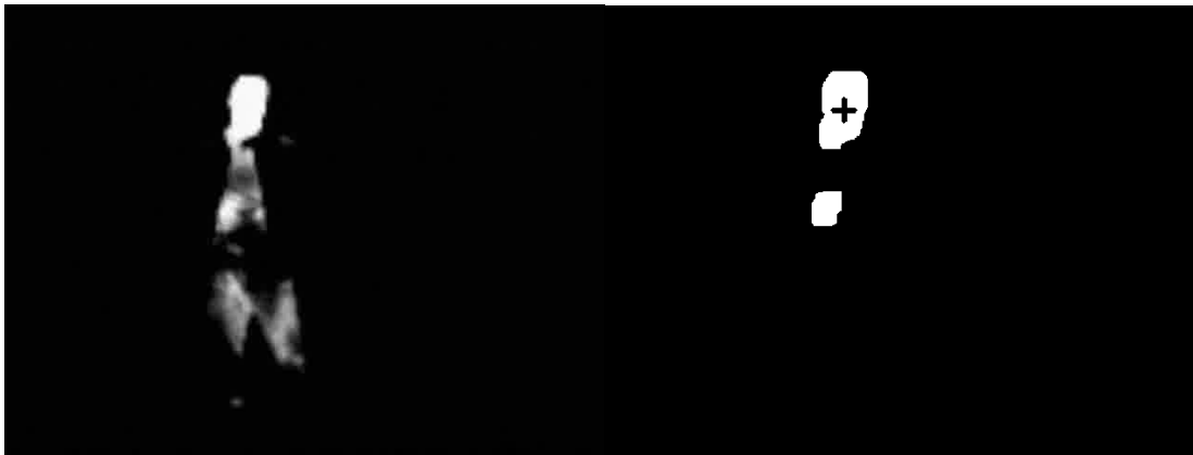
Figure 2: A segmented image (left) and centroid calculation (right).
