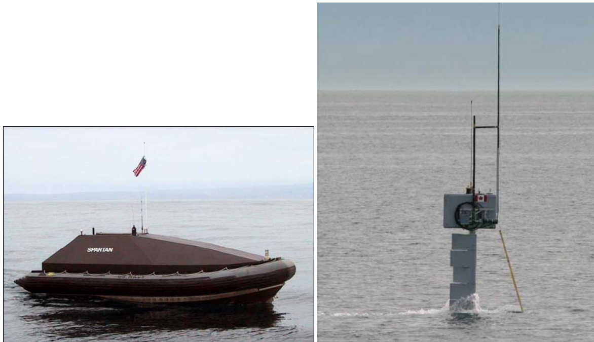
Figure 2.14: The Multi-Mission Spartan Vehicle (left) and the Remote Minehunting Vehicle Dorado (right) are Two Examples of Unmanned Surface Vehicles.
