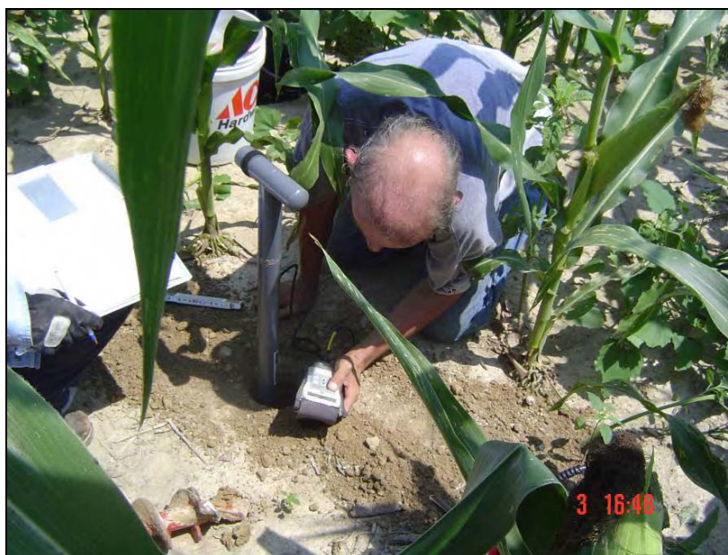
Figure D-1. Using ML2 and HH2 readout to measure soil moisture at depth within auger hole.
