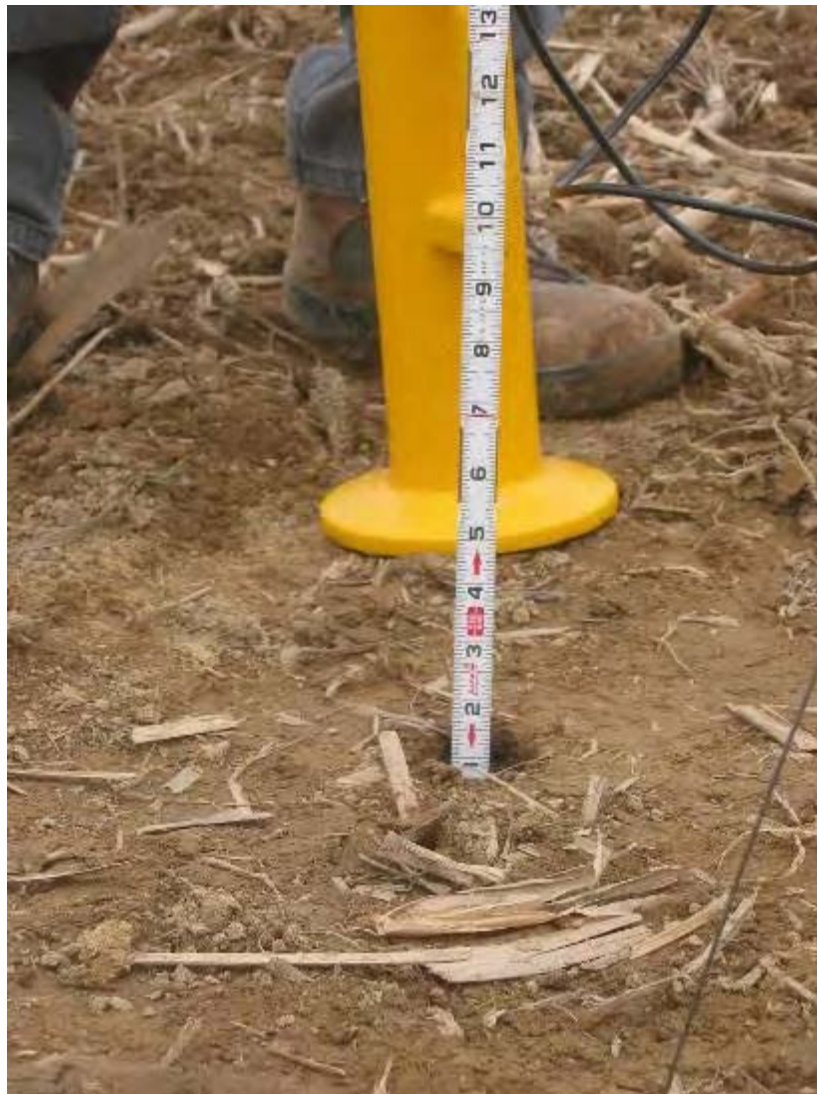
Figure 3-9. Typical indentation when attempting to use the standard (4.5-kg) Clegg hammer for upper soil strength measurements.
