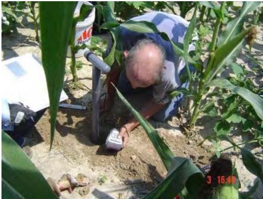
Figure 4-20. Taking soil moisture readings with a Dynamax ML2 in the auger hole (North Vernon Airport RAS, summer IOP2).
