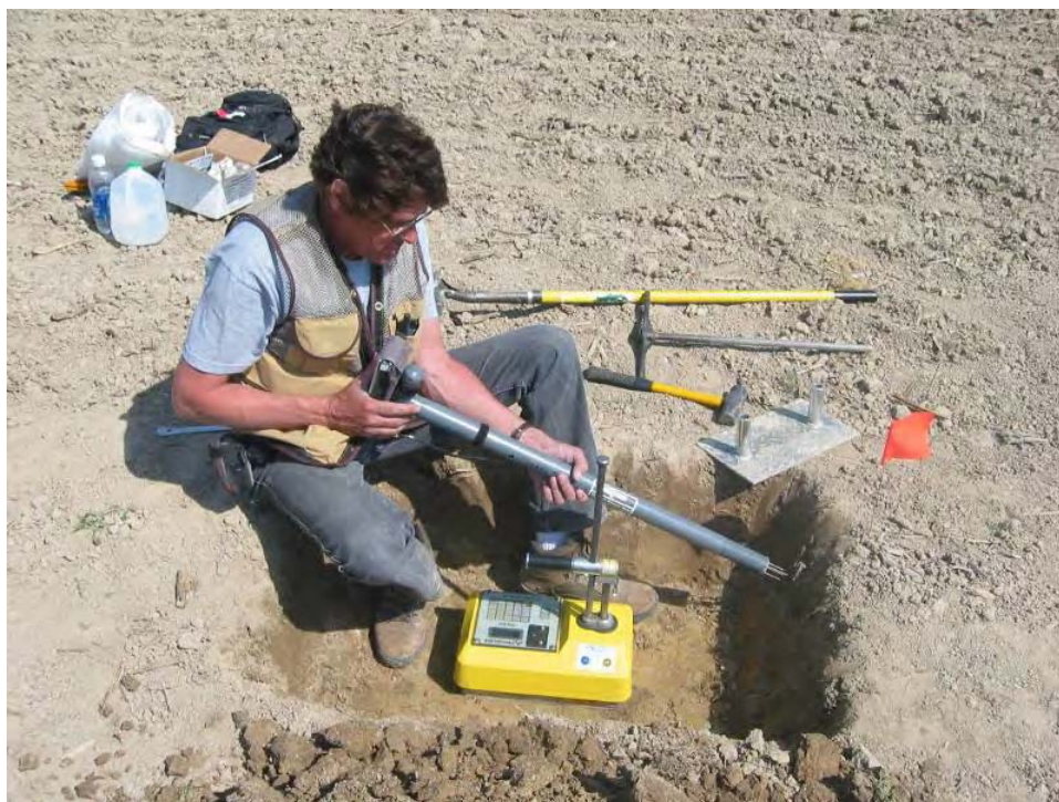
Figure D-4. Troxler nuclear gauge (yellow instrument) in moisture-reading configuration at the base of the soil pit. The Dynamax ML2 is held ready for measurement of soil moisture content, with the four stainless steel measuring rods visible at the right pit wall.
