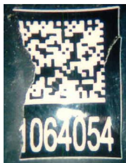
Figure 25. TESA Tape after Environmental Testing
