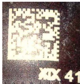
Figure 24. Laser Etch and Clear Coat after Hot, Cold and Icing
