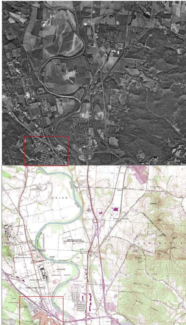
Figure 3-9: Comparison of 1:24000 map feature density to 1m resolution aerial photograph. Note that the reduced visual information on the map enables more rapid comprehension of key terrain and cultural features.
