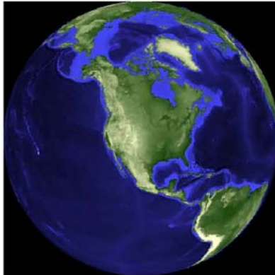
Figure 3-3: An orthographic projection rendering of the same ETOPO-5 data set with the projection centered on North America.
