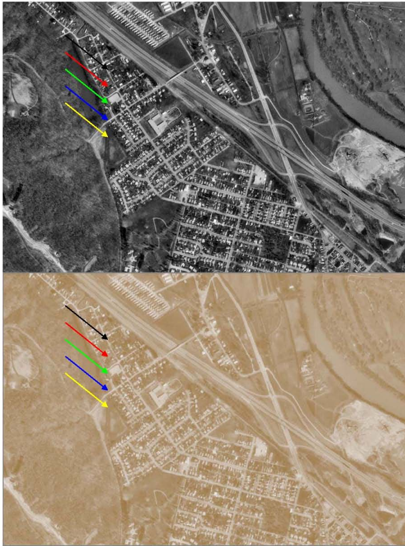
Figure 3-10: Reduced pallet rendering of photographic images improves legibility of overlays/symbols, using the image for spatial reference, not exploitation.
