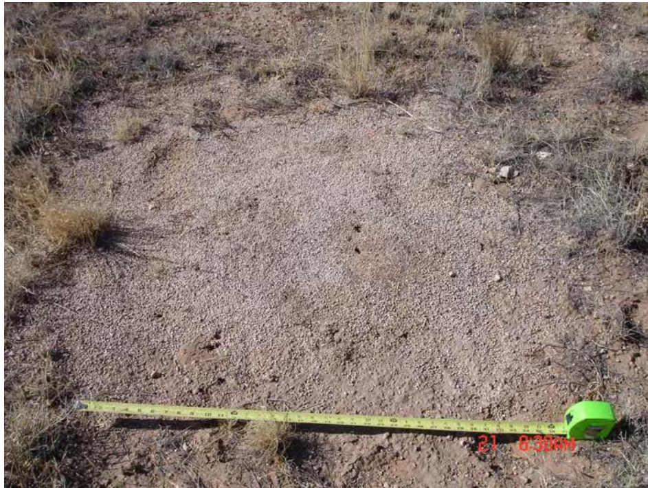
c. Example of a clear area with small holes and small caliche particles on the surface. Photo taken near station 8+20 during IOP #3.
