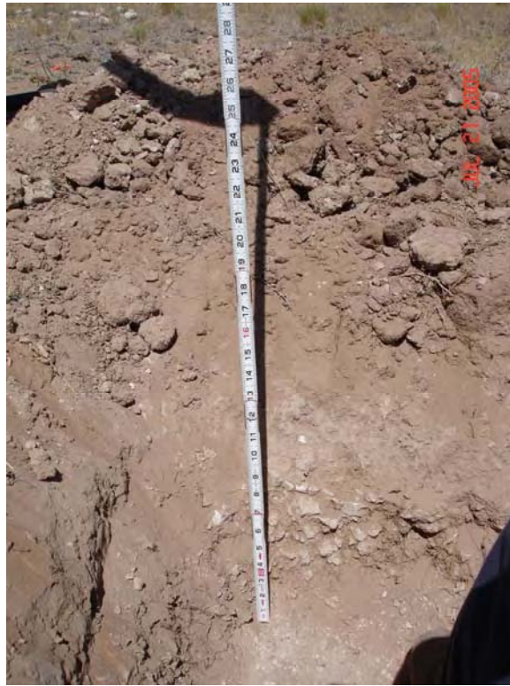
a. Entire soil pit where the bottom of the pit is located at 0.5 m (20 in.) below the surface.
