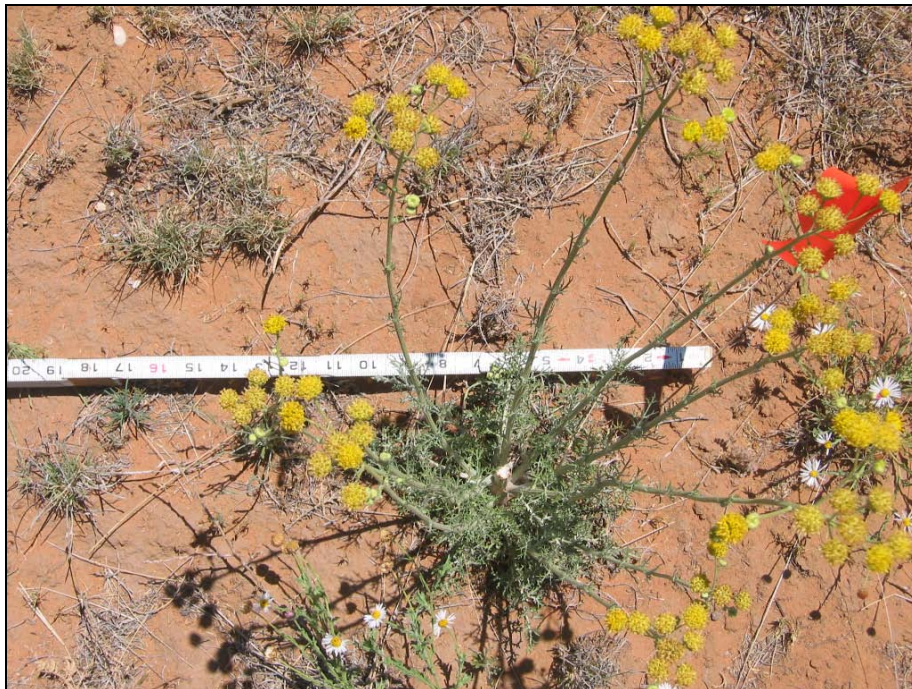
Figure A2-20. OLS 276-Short at start flag and undisturbed soil and vegetation condition on north side of flag. Munsell color chart 10YR 5/4. Field soil is identified as fine-grained soil (silty sand or silt) and a few pieces of gravelly material (caliche pieces). The soil is very dry.
