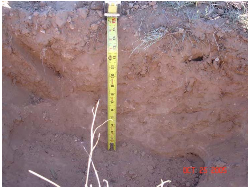
a. Soil pit down to 0.3 m (12 in.) below the surface.
