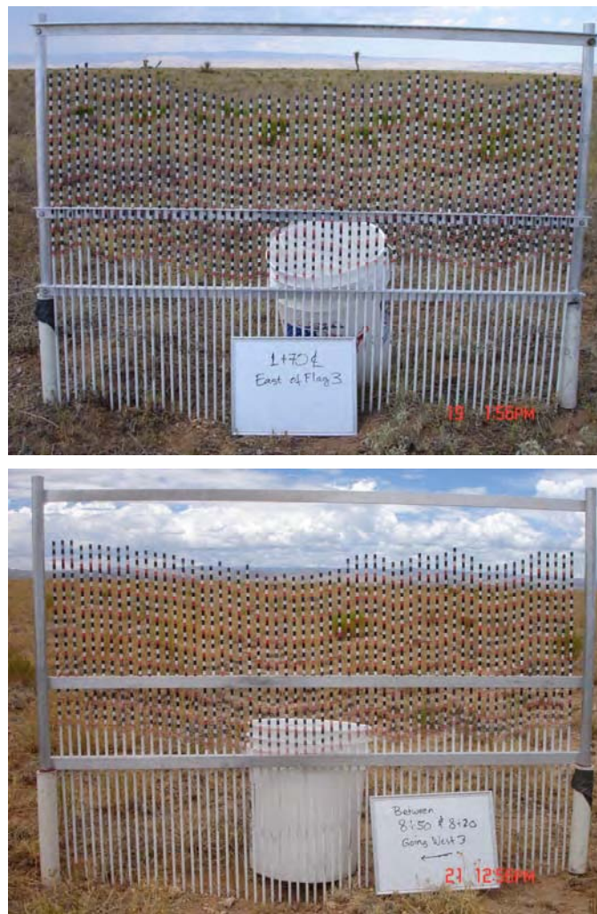
c. Surface undulation using the profilometer. The rods are horizontally spaced 2 cm apart and each rod is vertically marked at 1-cm intervals.
