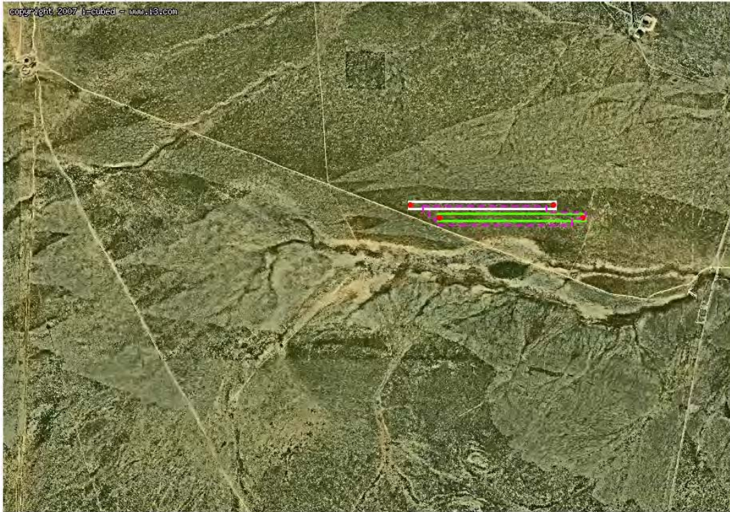
Figure 47. Shift on RAS location due to georectification level of imagery. Fort Bliss RAS Precision Corrected Imagery (PCI-RAS) in white and Systematic georeferenced (SI-RAS) in green. Field work was conducted at the SI-RAS. The magenta broken line shows the boundary of the clusters on OLSs in the area.
