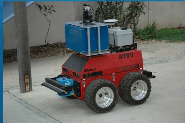
Space Micro Inc.: Autonomously detect, identify, and locate radiation sources
