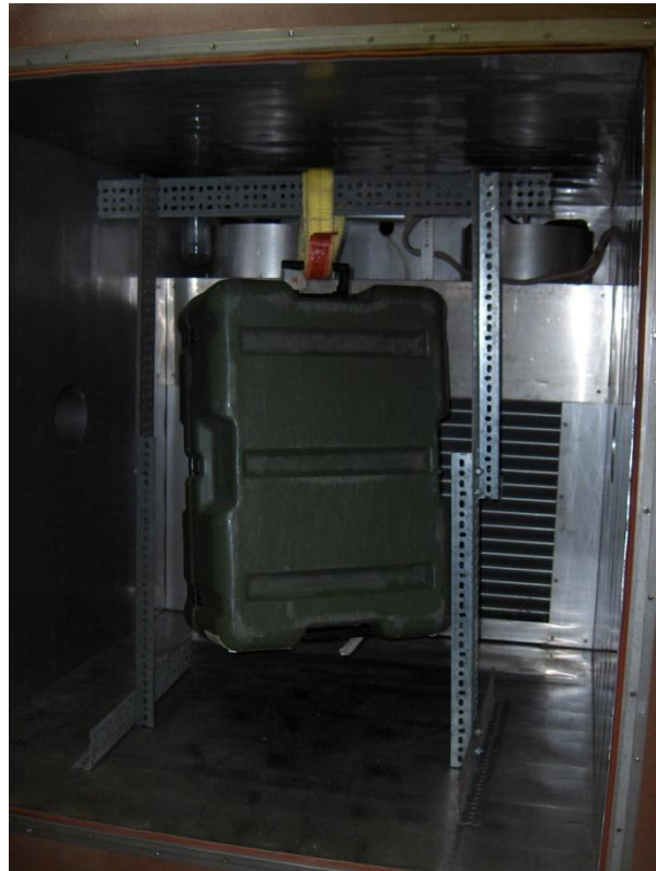
Figure 4. Handle strength test, hot.
