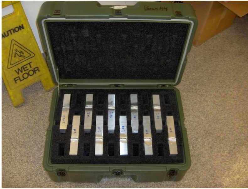
Figure 1a. Case with dummy loads inserted.
