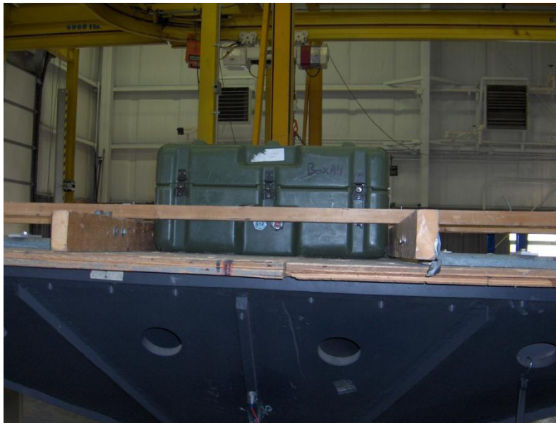
Figure 14. Loose load vibration test.
