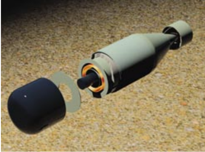
3-D computer mock-up of superconducting coil with core in torpedo housing.
