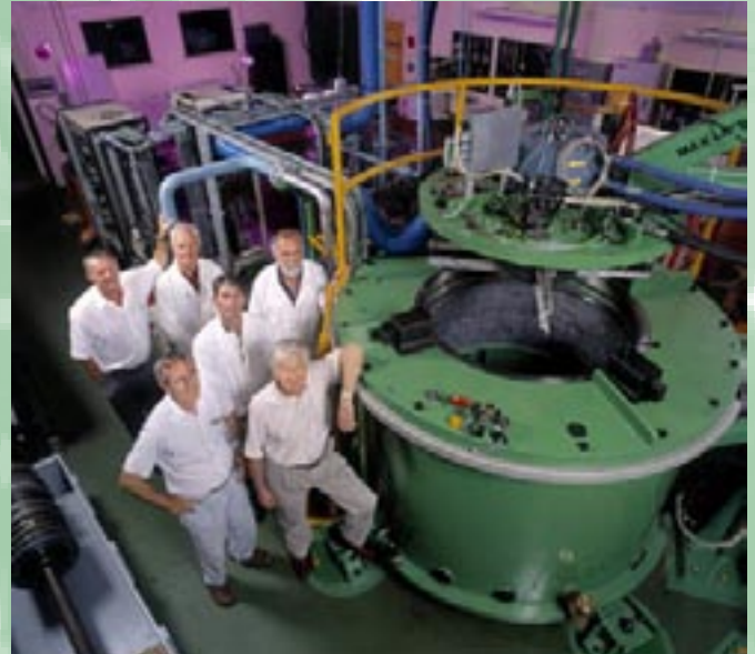
DSTO personnel with T56 spin test apparatus
