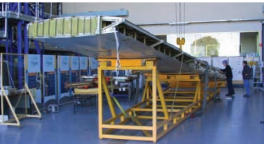
Orion wing under structural test.
