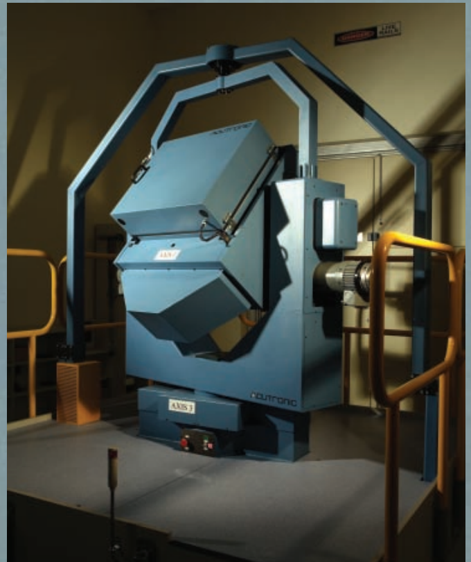
Above: Acutronic flight simulation table in stationary mode.
