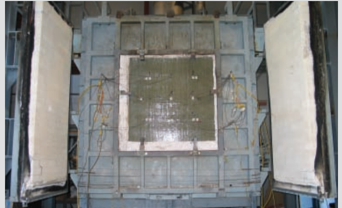
Apparatus for fire resistance testing at Werribee campus.
