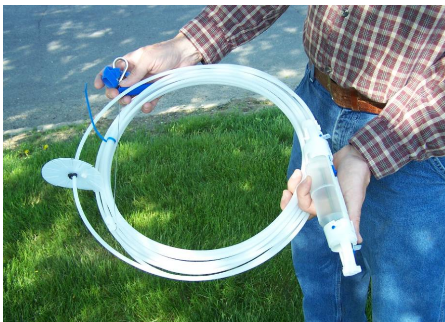
Figure 5. Snap Sampler trigger line with baffle.
