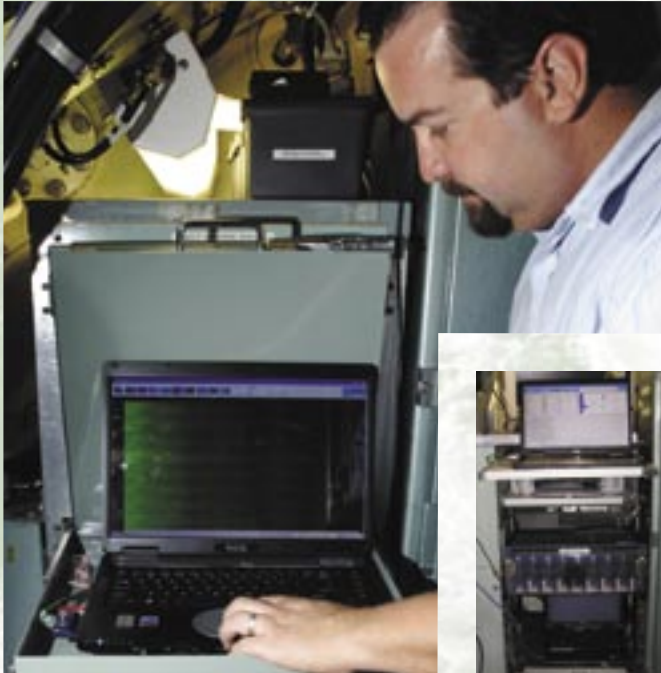
Wet Nurse submarine sonar diagnostics system.
