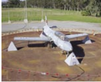
Aircraft being tested for electromagnetic effects using direct current injection techniques.
