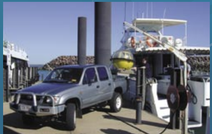
Wave rider buoy being loaded aboard vessel for deployment during radar surveillance trial.
