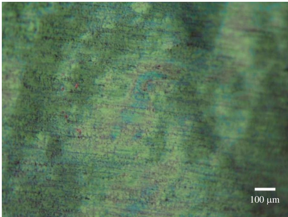
Figure 27. Optical Micrograph of AlON on Titanium Foil
