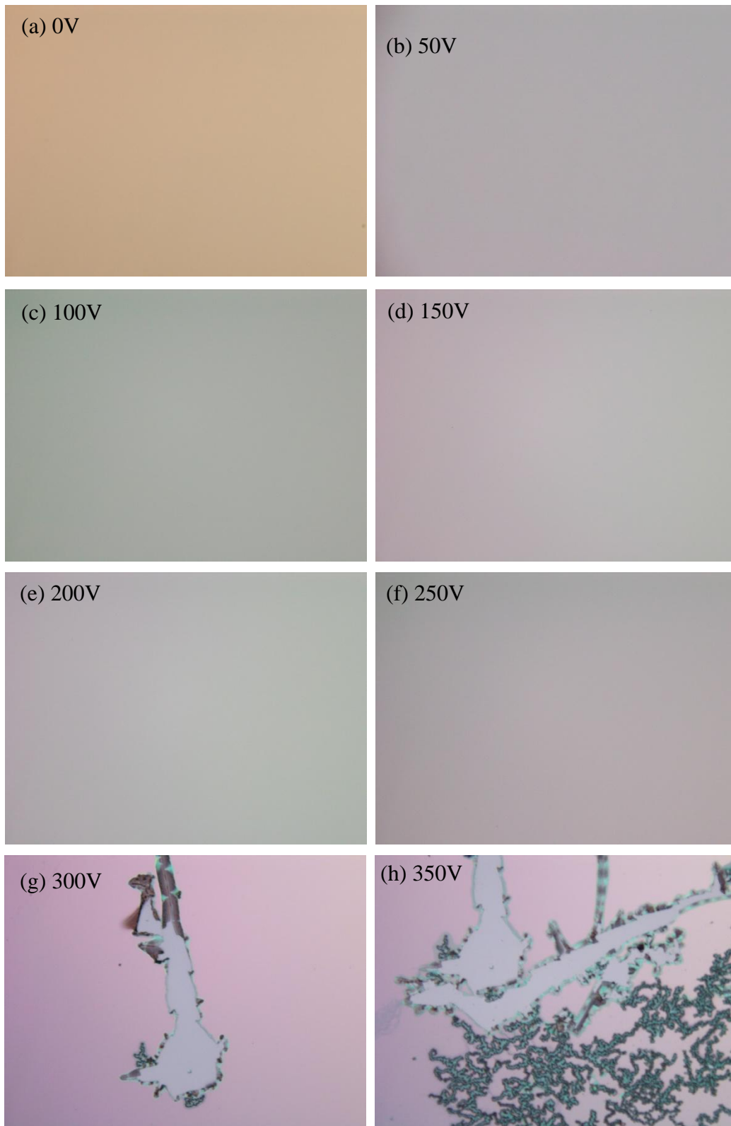
Figure 53. Optical Images of Capacitor Surface after Applied Voltage from 0 V to 350 V
