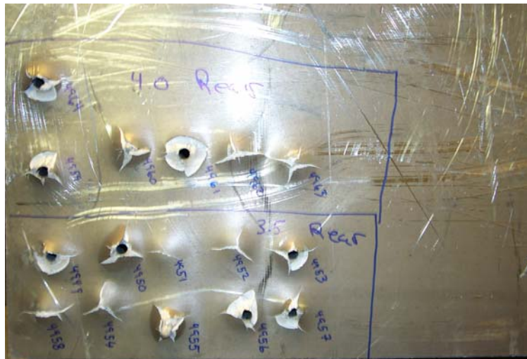
Figure A-6. The 3.5- and 4.0-in AZ31B-H24: 0.50-cal. APM2 impacts.
