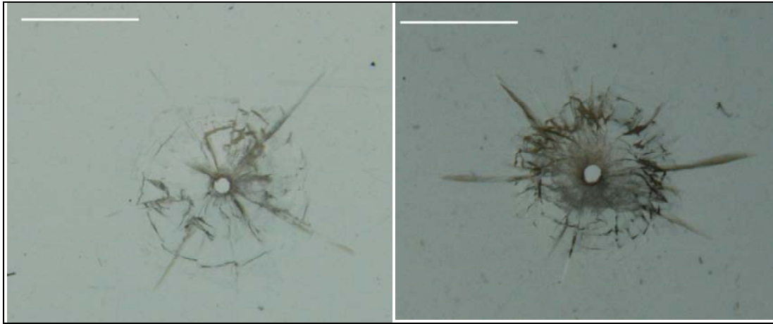
Figure 3. Damaged areas on targets: impact speed of 205 m/s (left) and impact speed of 250 m/s (right). The white scale bar is 3.5 mm.
