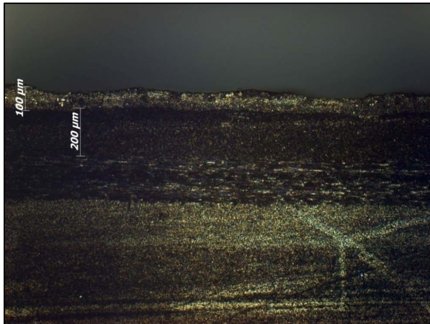
Figure 16. Configuration Ext (Exterior), 200 gsm nickel (note approximately 100μm nickel on external surface).
