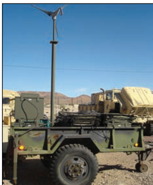
Figure 14: Transportable Hybrid Electric Power Stations (THEPS)
