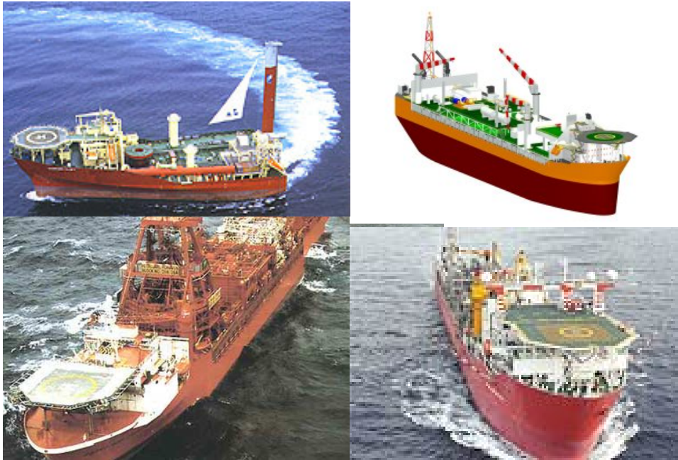
Figure 9 - Examples of Forward Helicopter Decks on FPSOs
