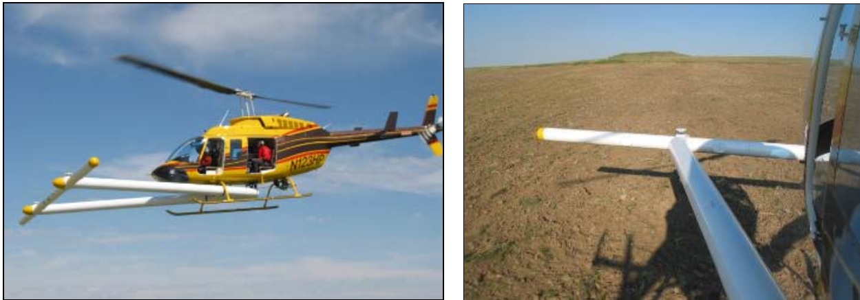
Figure 1. Helicopter MTADS Technology as Deployed on Bell Long Ranger Helicopter for Demonstrations at Pueblo, Kirtland and Victorville PBRs.
