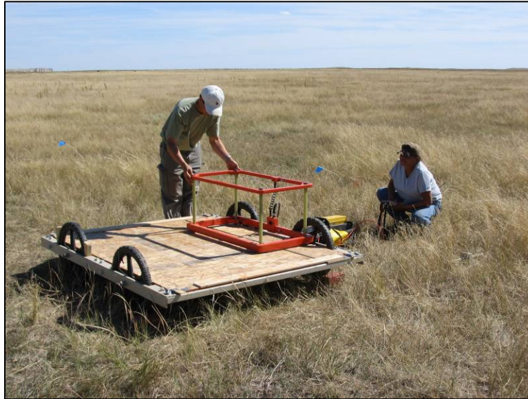
Figure 2. EM61 sensor during cued data collection.
