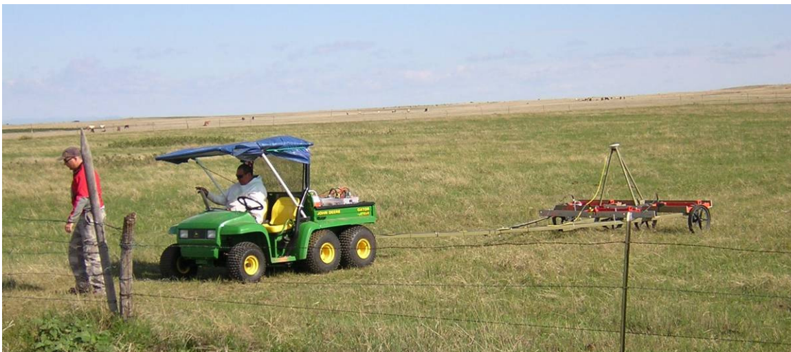
Figure 3. Parsons three-coil EM61 array deployed at the Badlands Bombing Range.
