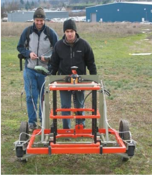
Figure 1. Modified EM-63 cart collecting discrimination mode data at the Ashland test-site. Positional errors are minimized By minimizing the level-arm between the RTS prism and the coil and including the IMU for orientation.
