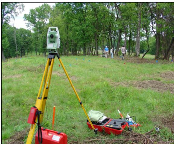
Figure 2. Sky Research utilizes the Leica RTS TPS1206 laser positioning system. This device is set up in over a known point and tracks a prism attached to the geophysical survey equipment.
