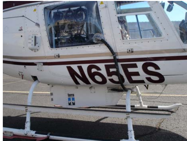
Sensor pod mounted below helicopter, control console visible through window.
