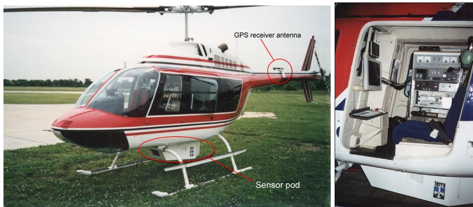
Figure 2-1 Helicopter-mounted Lidar and Orthophoto Sensor Equipment
