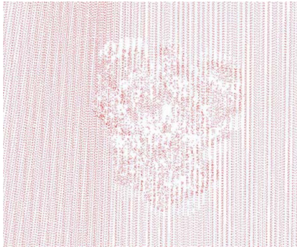
Lidar points, 450 m flight, showing different areas with few or no lidar points.
