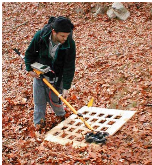
Figure 1: Collecting EM61-HH data on a grid over a suspected buried UXO item.
