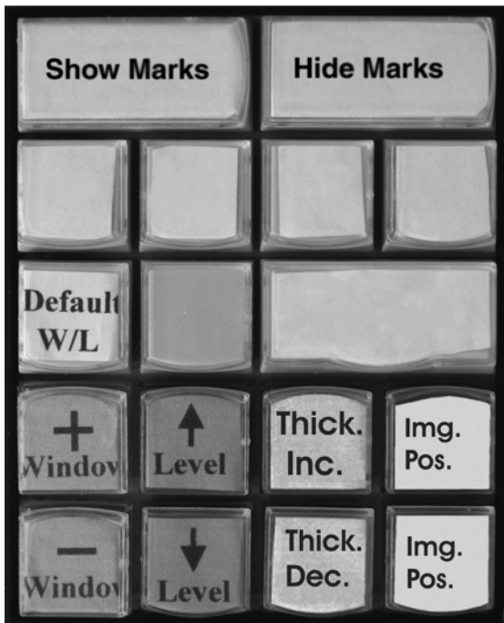
Figure 1: Programmable keypad with which user can control the main display features.
