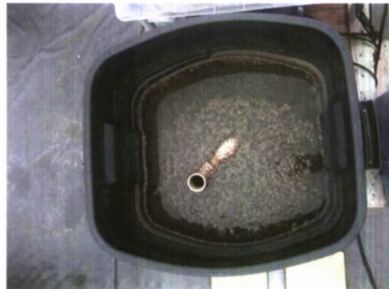
Figure 2-10. Top view of influent feed tank with mostly submerged standpipe shown.
