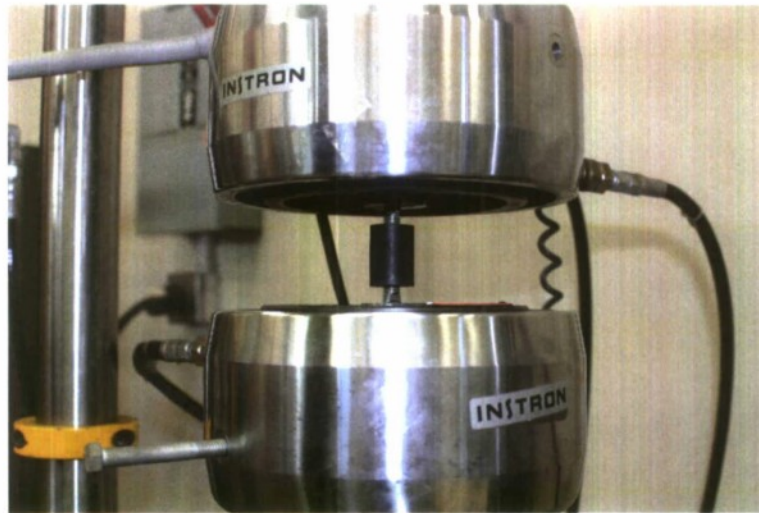
Figure 2.30: Overview of a specimen in the Instron uniaxial testing machine.
