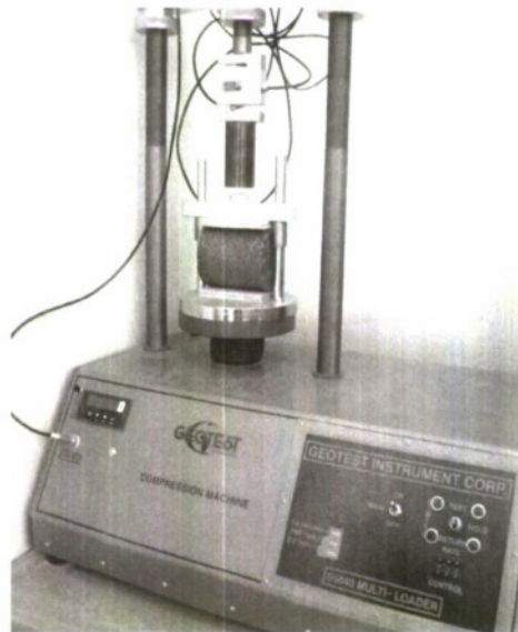
Figure 3. Machine used for ITS and UCS test
