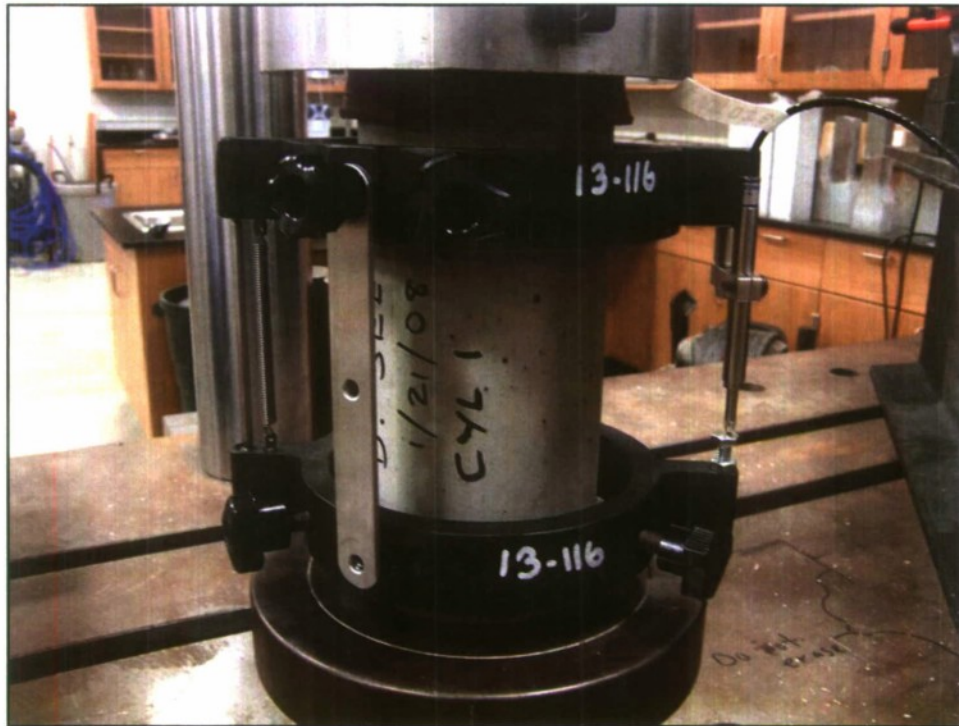
Figure 2: Capped Compression Specimen with Compressometer Fixture.
