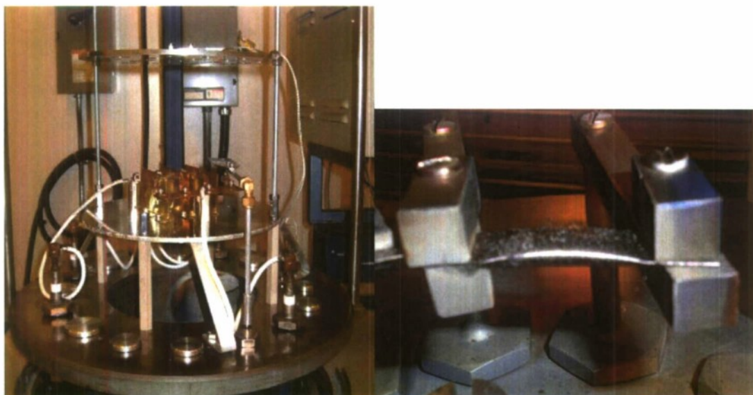
Figure 2. Left is a thermal vacuum evaporator. Used in depositing thin films. On the left is the crucible being held by two electrodes. Tungsten mesh is wrapped around the crucible to help keep the chalcogenide glass bulk material from flying out.
