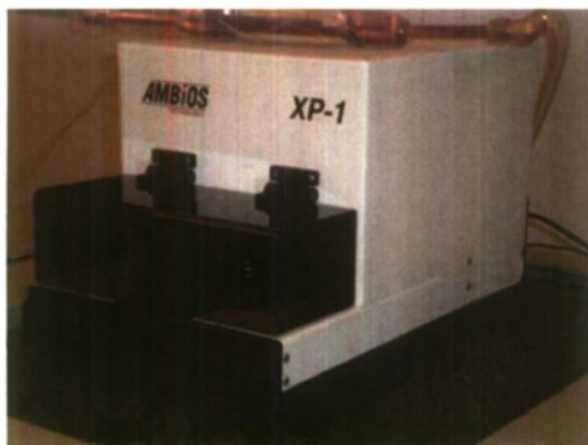
Figure 4. The profilometer that is used to measure thickness of the thin films.
