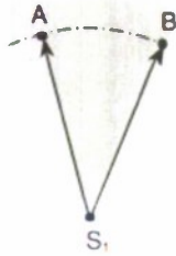
Figure 1 – Point A and B have the same scalar distance from a single ultrasonic sensor at S_1 and cannot be distinguished.
