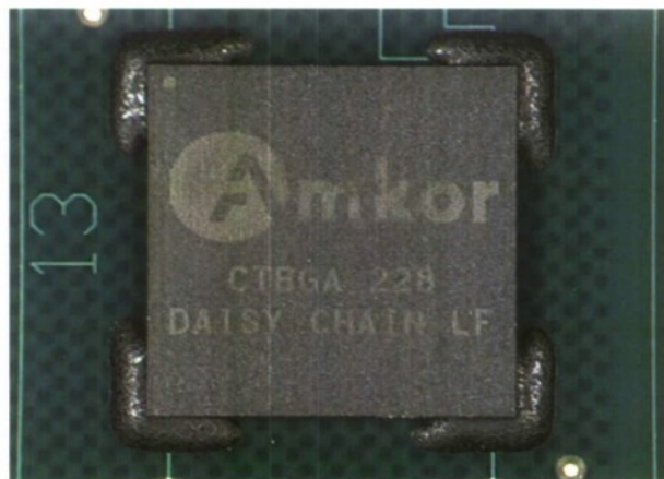
Figure 4. An edge-bonded CSP
