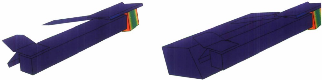
Figure 2.9: Comparison of fifth mode with and without support fixture.
