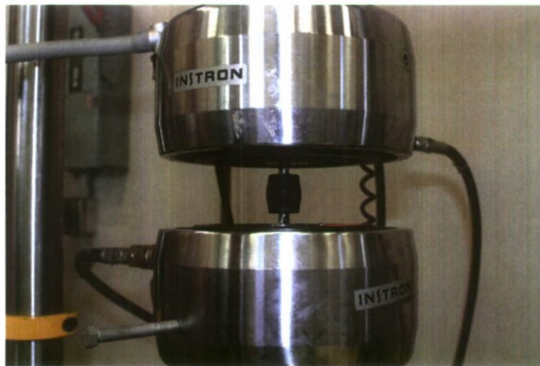
Figure 2.32: A specimen under uniaxial compression.
