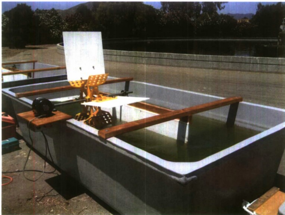
Figure 2-4. A high-rate pond tank during test filling, showing the central baffle, paddle wheel, and motor.
