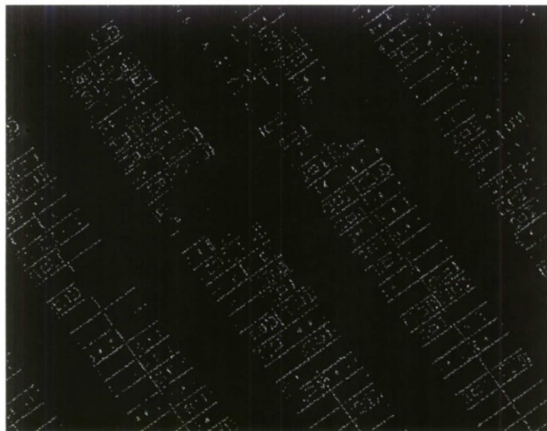
Figure 19: After a threshold of 200, the parking lot is ready for Hough processing.
