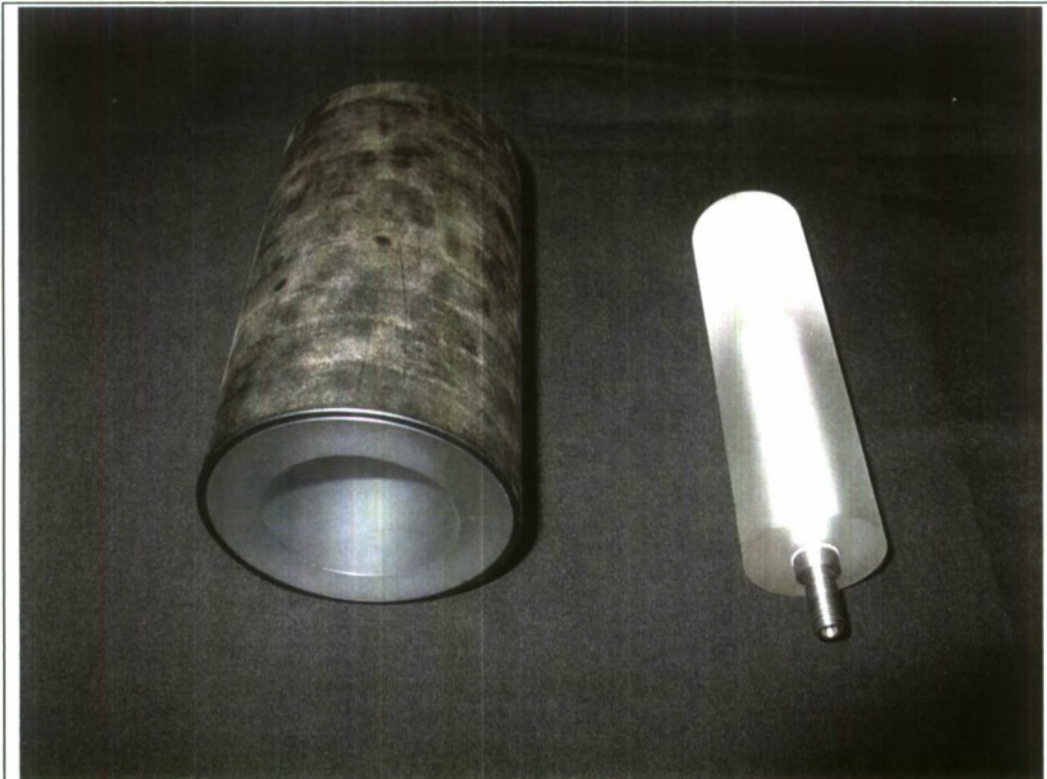
Fig. 8a. Inner and outer Plexiglas ® fuel grains that will form an annular combustion chamber.
