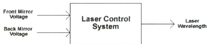
Figure 4.2 - Diagram of laser control system. Experimental setup for the ramped tuning feasibility experiment.
