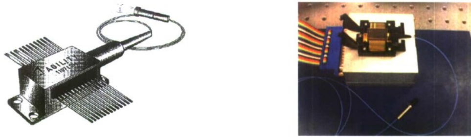
Figure 3.1 - The Agility 1107 laser. (Left) Packaged version of the Agility 1107 Widely Tunable Laser [13]. (Right) The image of the package version the Agility 1107 while used in the laboratory.
